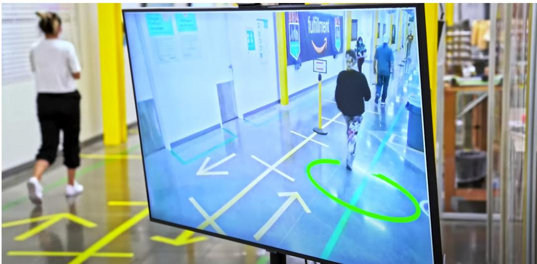
Amazon's Distance Assistant uses a 50-inch monitor, a camera, a local computing device and depth sensors to measure the distance between employees.
